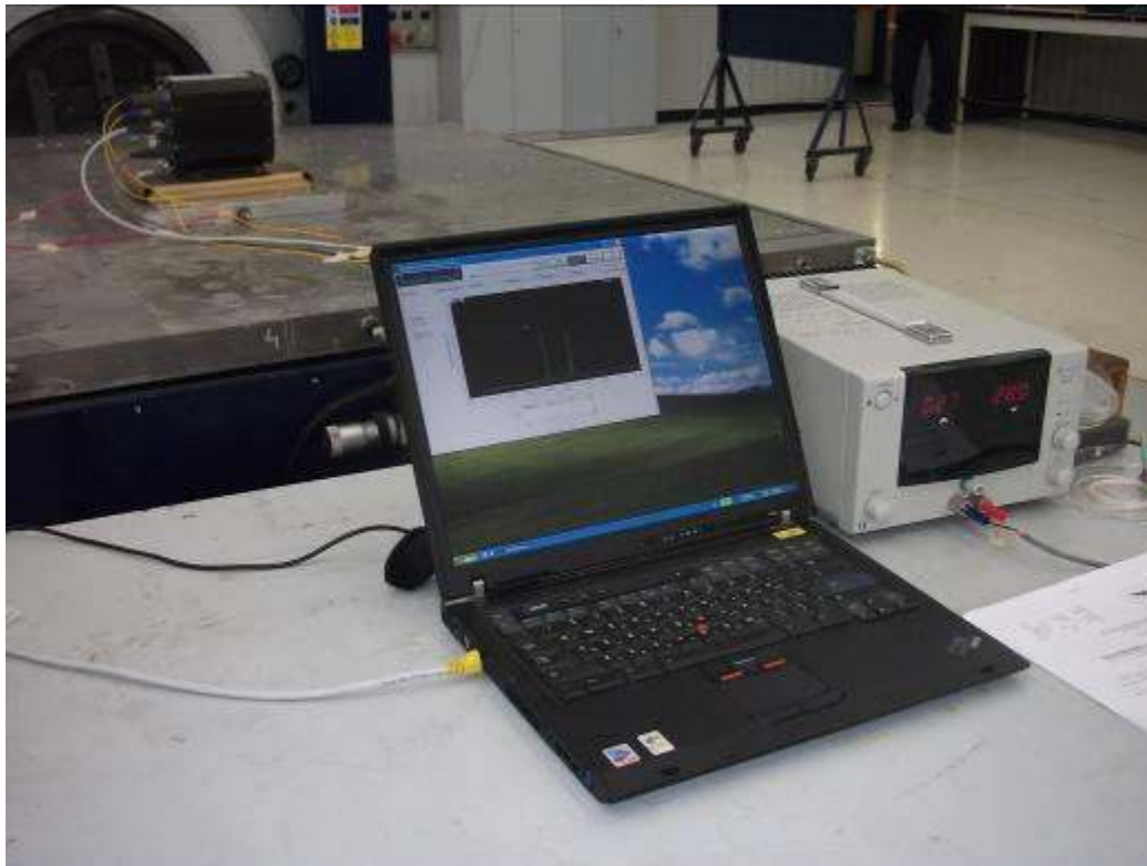
Photograph 2: Vibration and Shock Test setup – Y Axis Data recording of two channels
