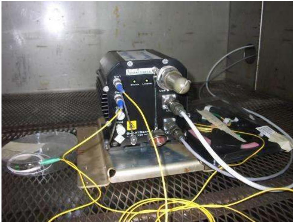
Photograph 4: Temperature - Altitude Test setup Date recording of two channels by USB disk
