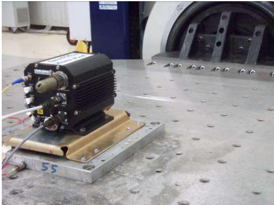
Photograph 3: Vibration and Shock Test setup – X Axis
