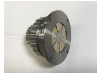
With magnetostrictive FBG proximity sensor
