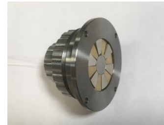
With magnetostrictive FBG proximity sensor
