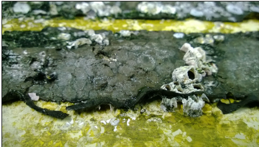
Fig. 5: Barnacles creeping under the protection layer of plate 37/38.
