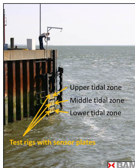
Fig. 1: Set-up of the test rigs with sensor plates in the three tidal zones
