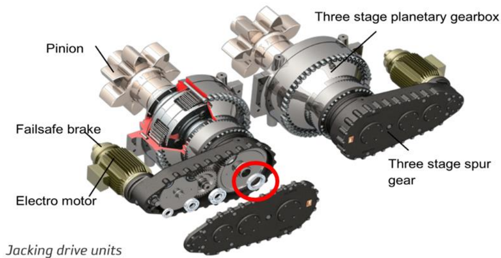
Figure 5: A typical jacking drive unit, starting with an electro motor, drives a four or three spur gearbox. Indicated by a red circle is the position of the fiber optic sensing bearing for static and dynamic load measuring in the jacking drive units [4].
