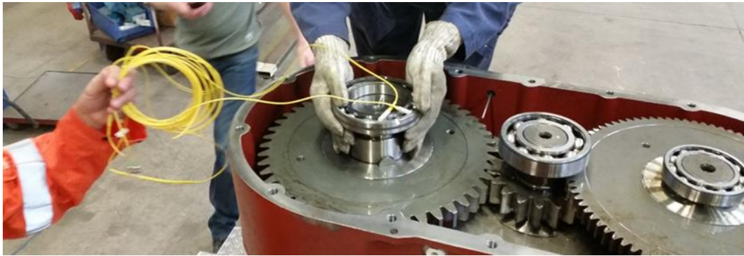
Figure 9: Installation of the fiber sensing bearing in the jacking system gearbox.
